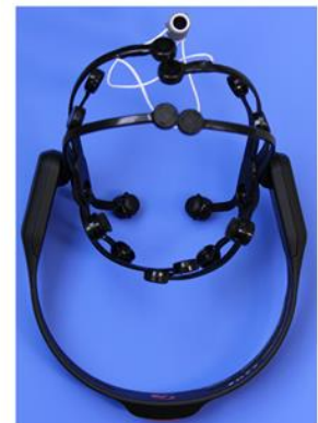
Figure 3: Brain-computer Interface (BCI) Setup Based on Electroencephalography (EEG) Signals.
